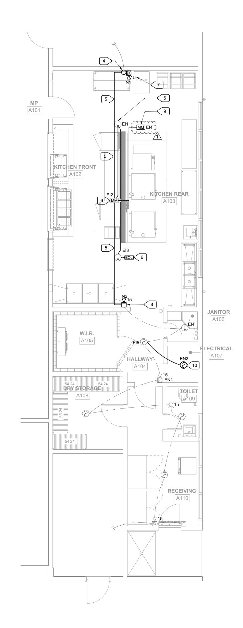
2 REMODEL FLOOR PLAN - FIRE ALARM
