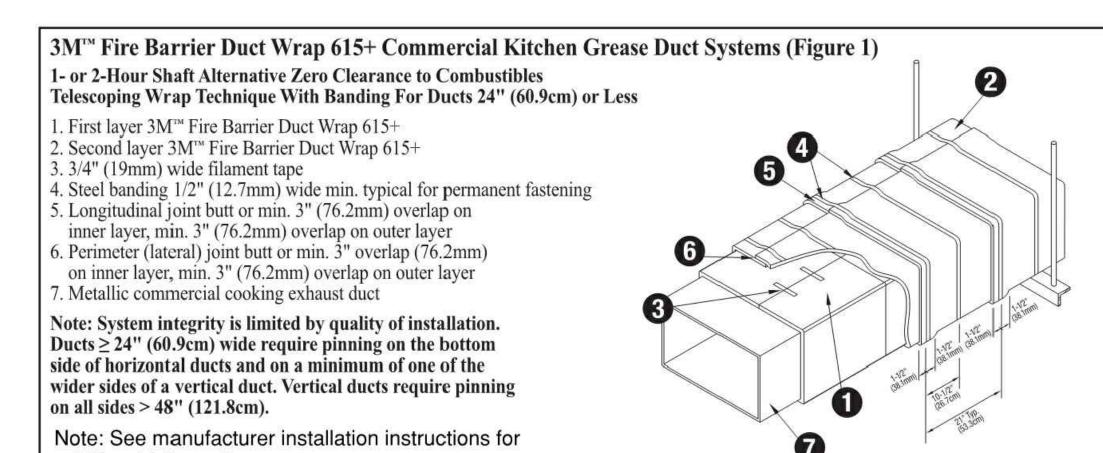
3M FIRE BARRIER DUCT WRAP 615+ CALIFORNIA STATE FIRE MARSHALL LISTING NO. 2440-0941:0112
