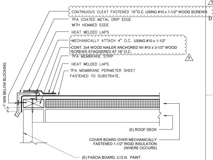
1) MAX. FACE DIMENSION SHOULD BE 5" TO PREVENT DISTORTION FROM "OIL CANNING." IF SURFACE DISTORTION IS ACCEPTABLE, FACE DIMENSION MAY BE INCREASED TO 8". 2) FOR FASCIAS GREATER THAN 8" INSTALL IN TWO SECTIONS.
