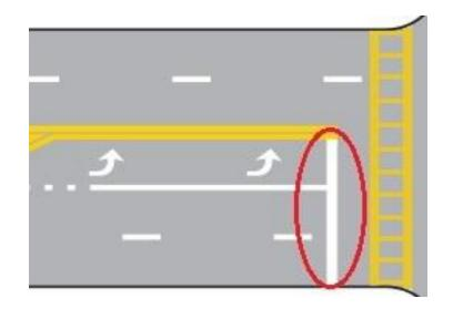
The oval highlights the stop line. A stop line is a solid white pavement marking line extending across approach lanes to indicate the point at which a vehicular stop is to be made.
