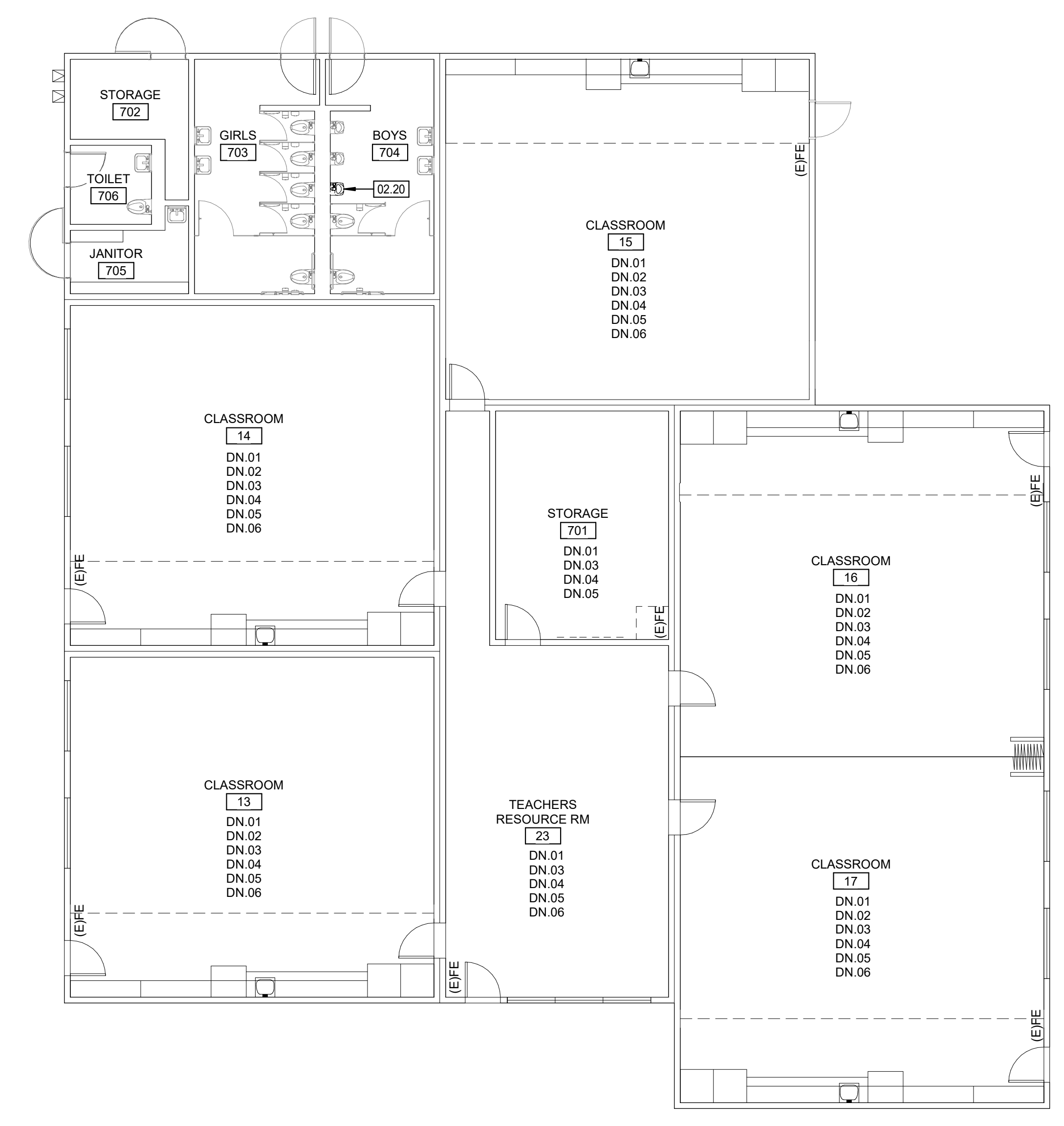
DEMOLITION FLOOR PLAN - BLDG 7 1 1/8" = 1'-0"
