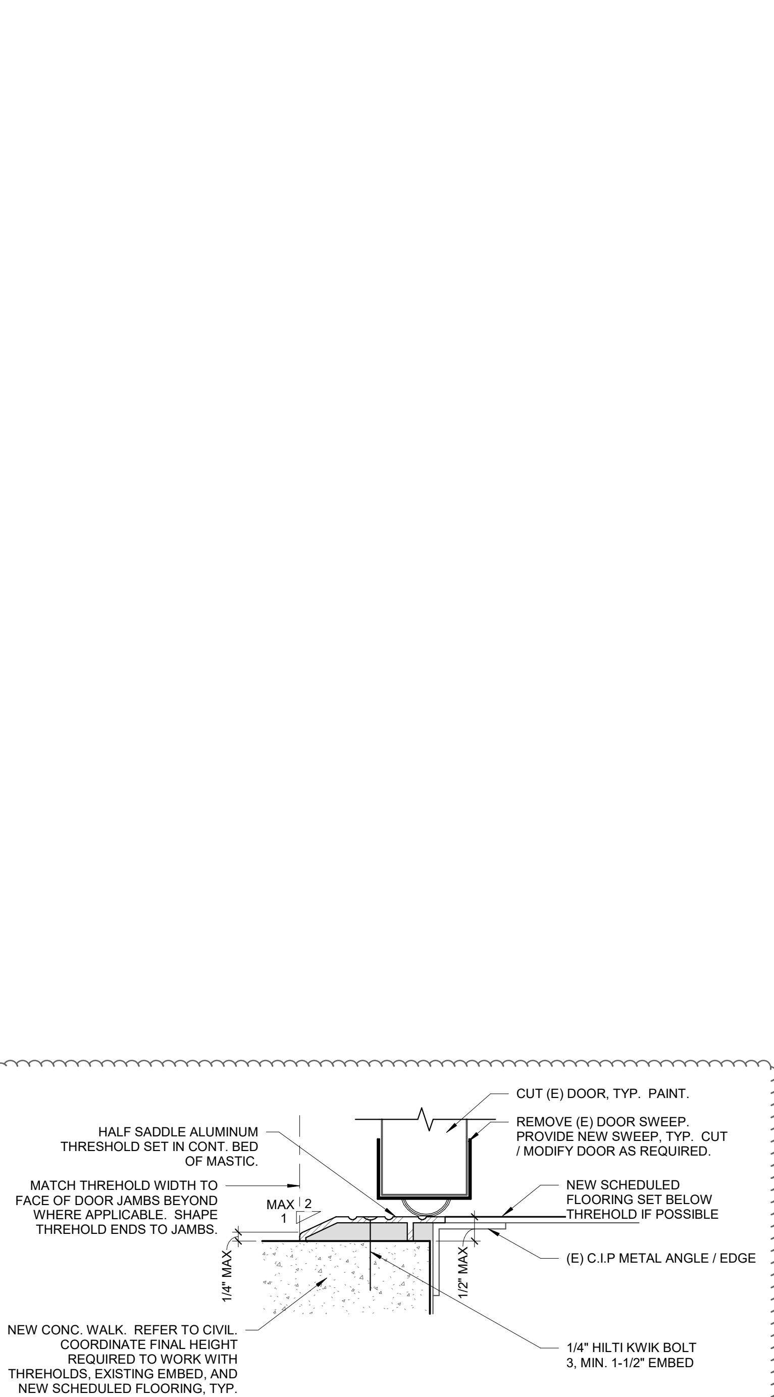
E6 THRESHOLD - HALF SADDLE 6" = 1'-0"
